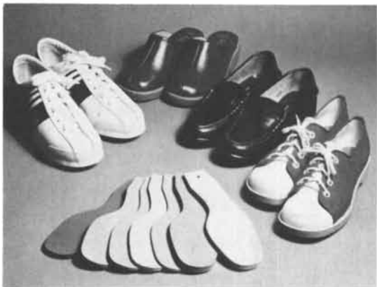
Photo III. Various kinds of cellular sponge shoe soles made of syndiotactic 1,2-polybutadiene
