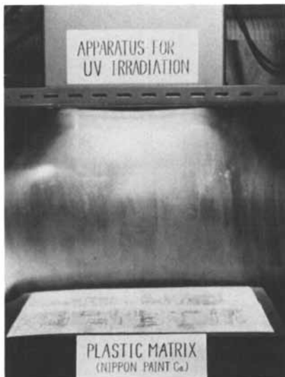
Photo V. The surface of the plastic matrix is photo-cured by UV irradiation
