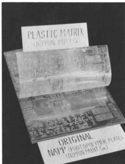
Photo IV. The plastic matrix (1,2-PBD) before UV irradiation is lifted from the master plate
