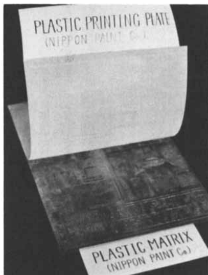
Photo VI. The relief images on the photo-cured matrix are transcribed to the printing plate (PP plate)
